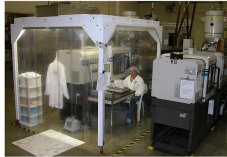
Hooded, Mobile Class 100,000 Cleanroom at Henry Plastic Molding
