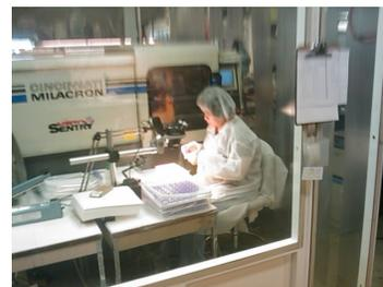
Class 100,000 Cleanroom in Operation at Henry Plastic Molding
